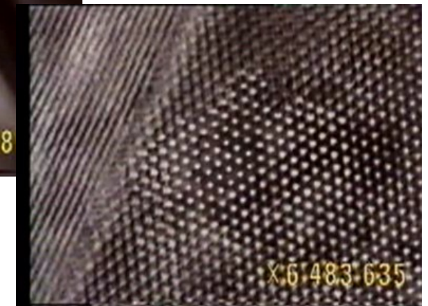
Structure atomique \text{Al}_2\text{O}_3 (0.1 nm)
